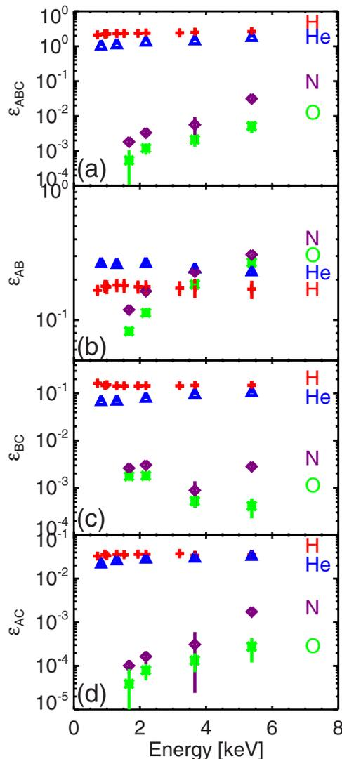
FIG. 2. (Color online) Detection efficiencies of H, He, N, and O for the (a)  $ABC$ , (b)  $AB$ , (c)  $BC$ , and (d)  $AC$  coincidence types.
