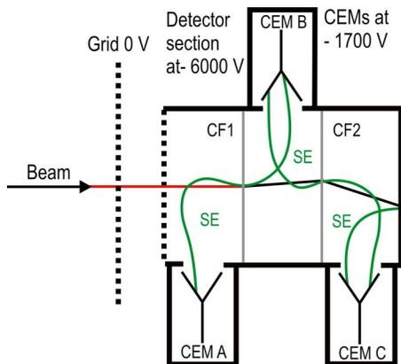
FIG. 1. (Color online) Schematic view of the IBEX-Hi detector as mounted in the vacuum chamber for testing.
